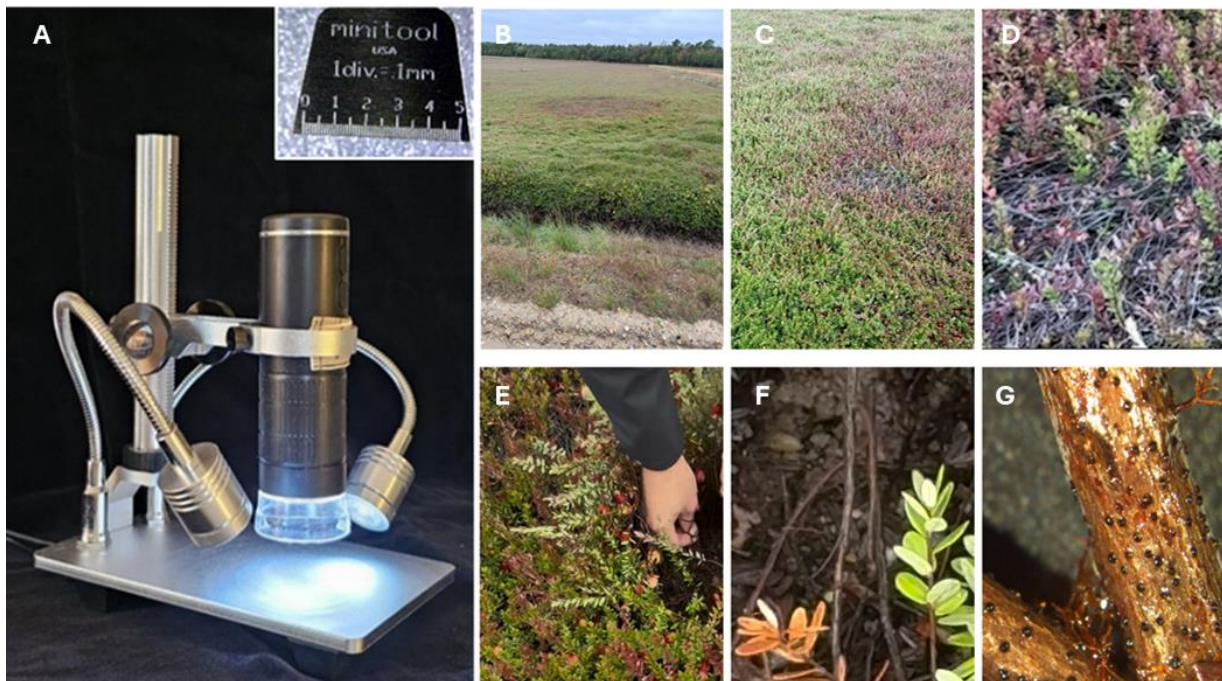
Fig 1. From Initial Detection to Verification. Simple digital microscopes are available from a variety of manufacturers. In this project we will use the Jusion WiFi/USB Digital Microscope the inset shows a 5mm scale bar with resolution to less than 0.1mm (Fig. 1a). It is advertised to be capable of 50 to 1000x magnification and is compatible with iPhone, iPad, Android, Mac, Windows and Linux. Ring-like structure observed from a field view (Fig. 1b); Edge of region showing fungal appearance inside the boundary (Fig. 1c); High magnification (50x) inspection of potential fungal region showing leaf discoloration, bare runners/stems (Fig 1d). Current practice of manually inspecting stem/stolon (Fig 1e); Stem appearance in camera image; Fig. 1f) Stem appearance in field microscope with dark spots confirming fungus (Fig 1g).
