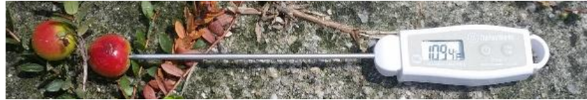
Fig. 3. An inexpensive meat thermometer being used to probe the internal berry temperature of a cranberry.
